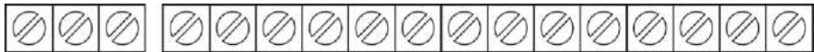
FWD REV S1 S2 S3 S4 GND FW FIC 10V FIV GND MCM
